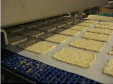
Filling mass's needs to float and amount of particles can't be bigger then 50% of the total substance. (Depending on substance/mass can the machine be equipped with pressure rollers and special wire cutters)
