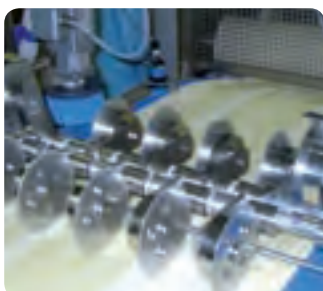
Strip cutting on the inlet conveyor
